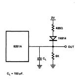
Figure 16. Test Load Circuit
